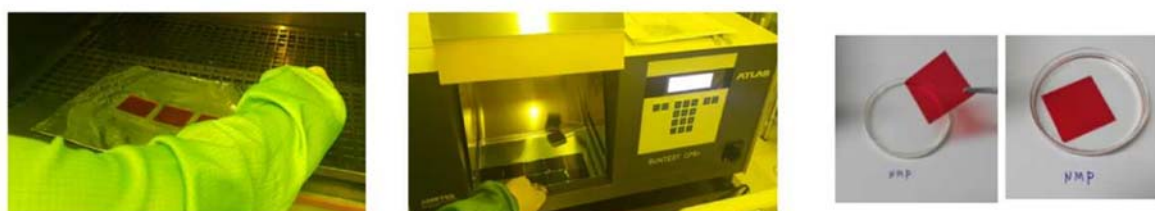
Fig. 3 : A light-fastness and solvent resistance test of DPP pigment
